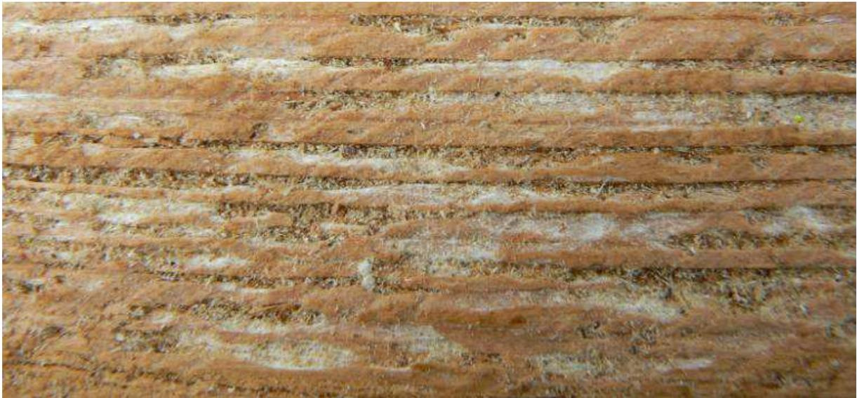
Fig. 2. The Scots pine's longitudinal section on the 3.5 m height. View characteristic for non selective delignification: dark color of lignin on which variform lumens filled with white cellulose were visible.
