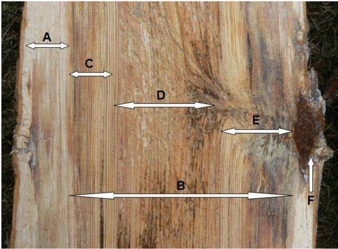
Fig. 4 The Scots pine's longitudinal section on the 13.0 m height: A – sapwood, B – heartwood, C – early decay, D – late decay, E – place of branch occurrence, dark colored area steeped with resin, F – dark colored slotted area filled with brown mycelium (the “blind” fruit body).
