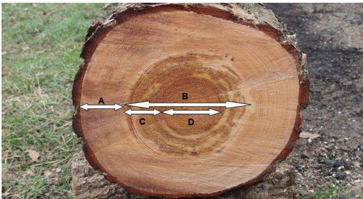
Fig. 1. The Scots pine's cross section on the 3,20 m height. By arrows there were tagged: A – uninfected sapwood, B – infected heartwood, C – early decay, D – late decay. Area infected by the early decay is covered with characteristic darker crescent pattern – the effect of lignin decomposition.
